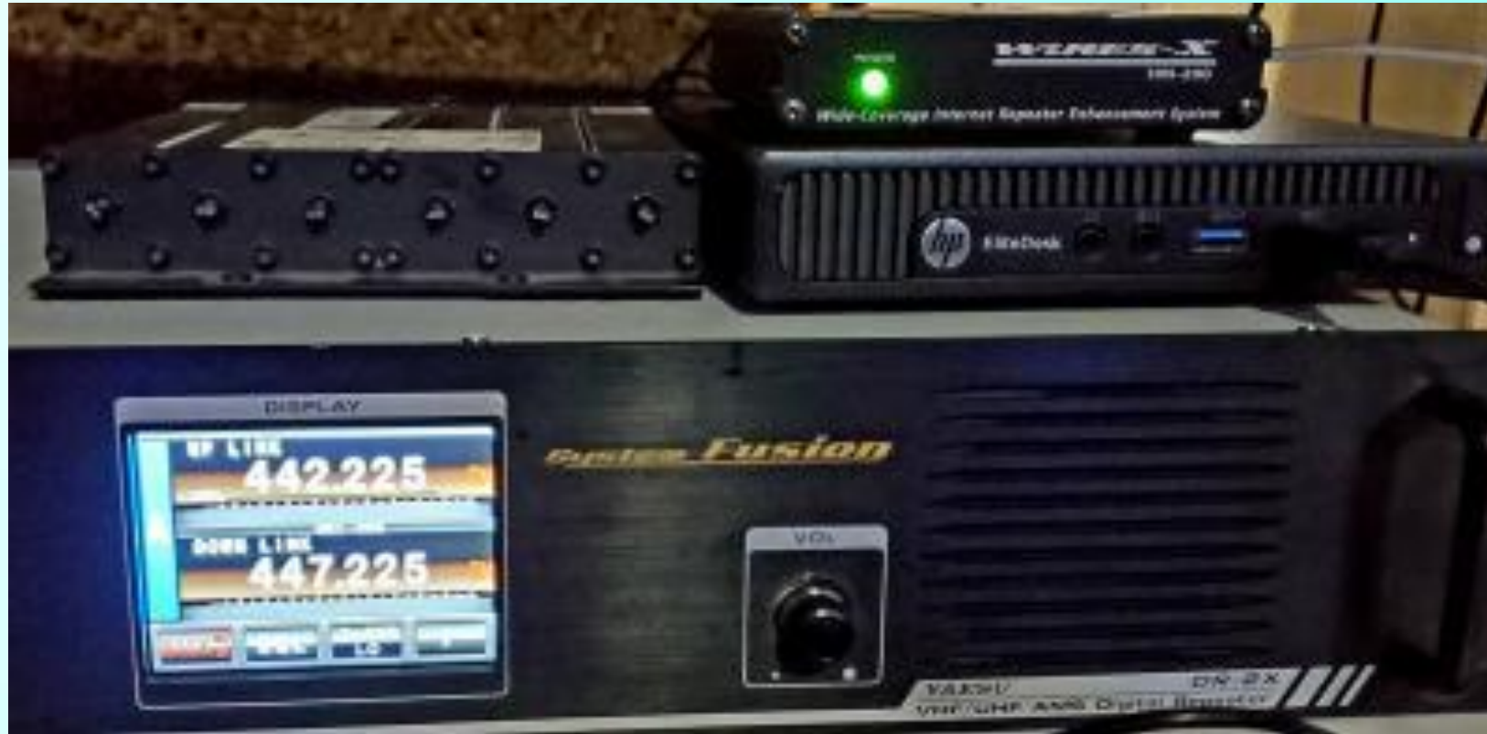
Yaesu System Fusion repeater with a n HRI-200 WiRES-X interface, a PC, and an Internet connection
